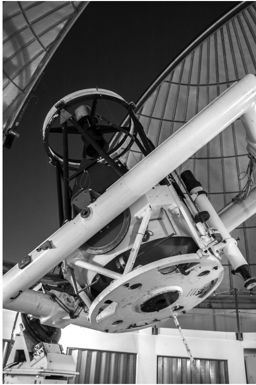
Figure 3.3. Catalina reflecting telescope on an equatorial mount. Camera at prime focus. Cassegrain focus is covered.
